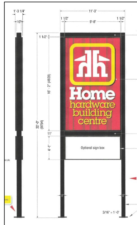
Figure 3 Pylon sign drawing submitted by the applicant.
